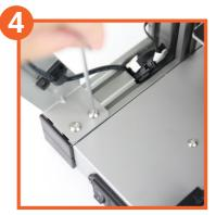
Inserting the block into the Right side aluminum slot and twist the bolt to lock it.
