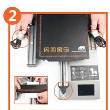
Remove the protection foam and tape from position.
