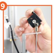
Install the filament sensor onto the cardan joint by one M3 **x 8mm** bolt. Then install the cardan joint onto the filament stand by one **M3 x 8mm** bolt.
