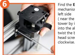
Find the **E1** extruding mechanism. Install it onto the ( near the Z axis screw) of tower by inserting the block into the aluminum slot and twist the bolt Mushroom head screw M4 x 5mm
