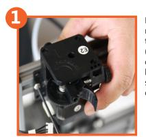
Find the **E2** extruding mechanism. Install it onto the right side ( on the other side of **E1**) of tower by inserting the block into the aluminum slot and twist the bolt clockwise.
