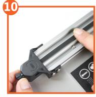
Twist the X axis belt tension adjusting knob clock wise to tighten the belt tension. You can check the tension by use one finger to push the belt. Either too tight or too loose would be perfect.
