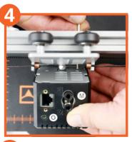
Install the printing head onto the gantry. Then to lock the head with 2 M3 x 6mm locking screw.
