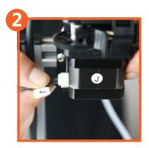
Insert the J male connector onto the J female Motor connector.
