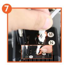
Insert the N tube into Nconnector.
