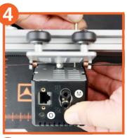
Install the printing head onto the gantry. Then to lock the head with 2 M3 x 6mm locking screw.
