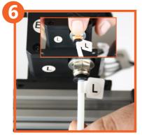
Insert the L filament tube into the L feeder. Then insert the orange locker to stop tube from falling out.
