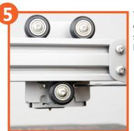
To push the printing head gently to ensure well secured. If not, re-lock the bolts.
