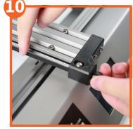
Twist the X axis belt tension adjusting knob clock wise to tighten the belt tension. You can check the tension by use one finger to push the belt. Either too tight or too loose would be perfect.
