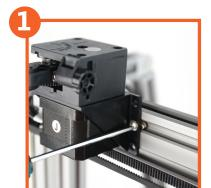
Find the **E2** extruding mechanism. Install it onto the right side ( on the other side of **E1**) of tower by inserting the block into the aluminum slot and twist the bolt clockwise.
