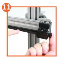
Twist the Y axis belt tension adjusting knob clock wise to tighten the belt tension. You can check the tension by use one finger to push the belt. Either too tight or too loose would be
