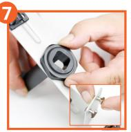
Install the filament plastic holder onto the left stand and twist the nut to lock it. Then install the 2 M3x 6mm bolts with the
