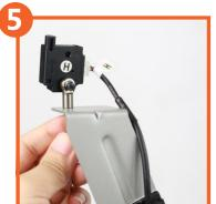
Install the filament sensor H onto the cardan joint by one M3 x 6mm bolt. Then install the cardan joint onto the filament stand by one M3 x 6mm bolt.
