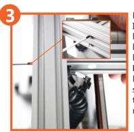
Put the printer base on it's side. Install the printer tower onto the base. Then use 4pcs M5 x 40mm bolt to lock the tower onto the
