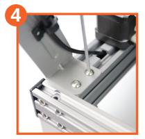
Inserting the block into the Right side aluminum slot and twist the bolt to lock it.
