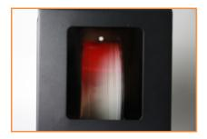
After you notice that the LED light turns red, the heating starts. You can dehumidify the filament alone, or you can heat it while printing.
