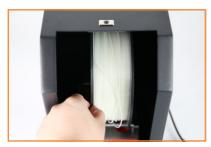
Put your prepared filament into BOX2,materials 3D printers using standard filament sizes:
